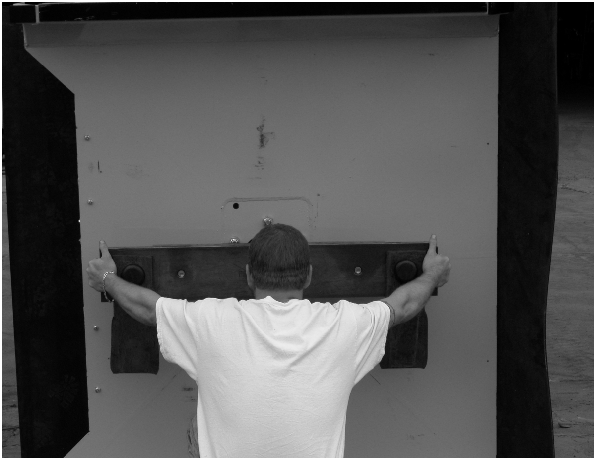
Fig. 2 Checking pre-load of the spindle housing bearings
